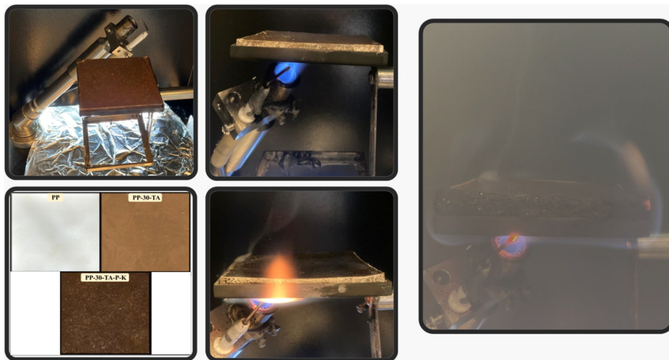
Figure 10. Images of PP composite samples exposed to a gas burner during the smoke density test.
